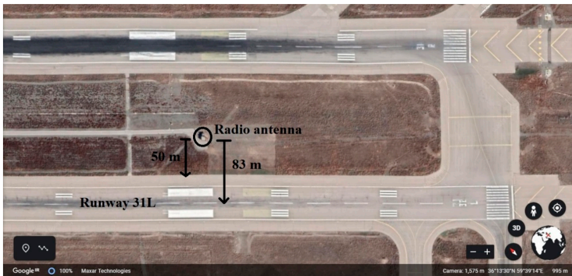
Figure 32. The exact location of the Radio antenna relative to runway 31L.
